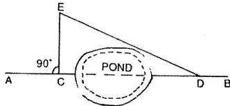
If the chainage of C= 50m and the distance CE= 40m, Find the chainage of D considering the angle CED= 30°. (5 marks)
